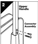
Slide upper handle section over matching section of the connector assembly. Insert short screw into top hole and long screw into the bottom hole then tighten firmly until handle is no longer loose.
